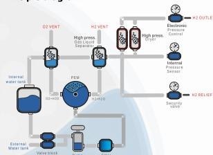
Hydrogen is produced from distilled water using a polymeric membrane (PEM). No acid or alkaline solutions are used.
