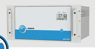
The RACK.WM series generators use an electrolytic cell with polymeric membrane (PEM) to produce pure hydrogen. The innovative gas drying system is completely maintenance-free and allows continuous operation, 24 hours a day. The exclusive, electronically-controlled gas/liquid separator, automatic checking for internal leaks whenever starting the unit, and constant control of operating parameters guarantee maximum safety. Up to 20 units can be connected in parallel.
